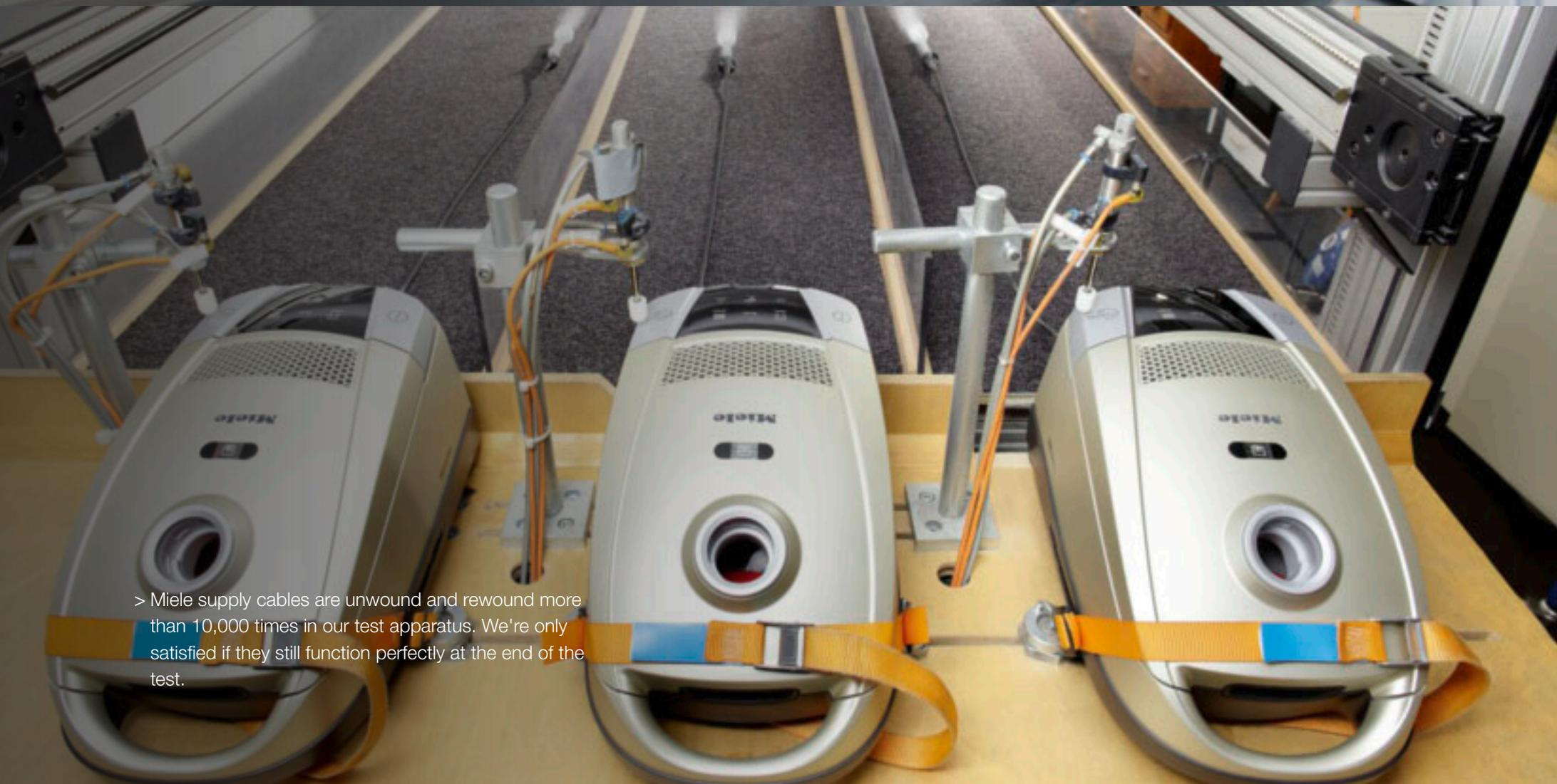
> Miele supply cables are unwound and rewound more than 10,000 times in our test apparatus. We're only satisfied if they still function perfectly at the end of the test.
