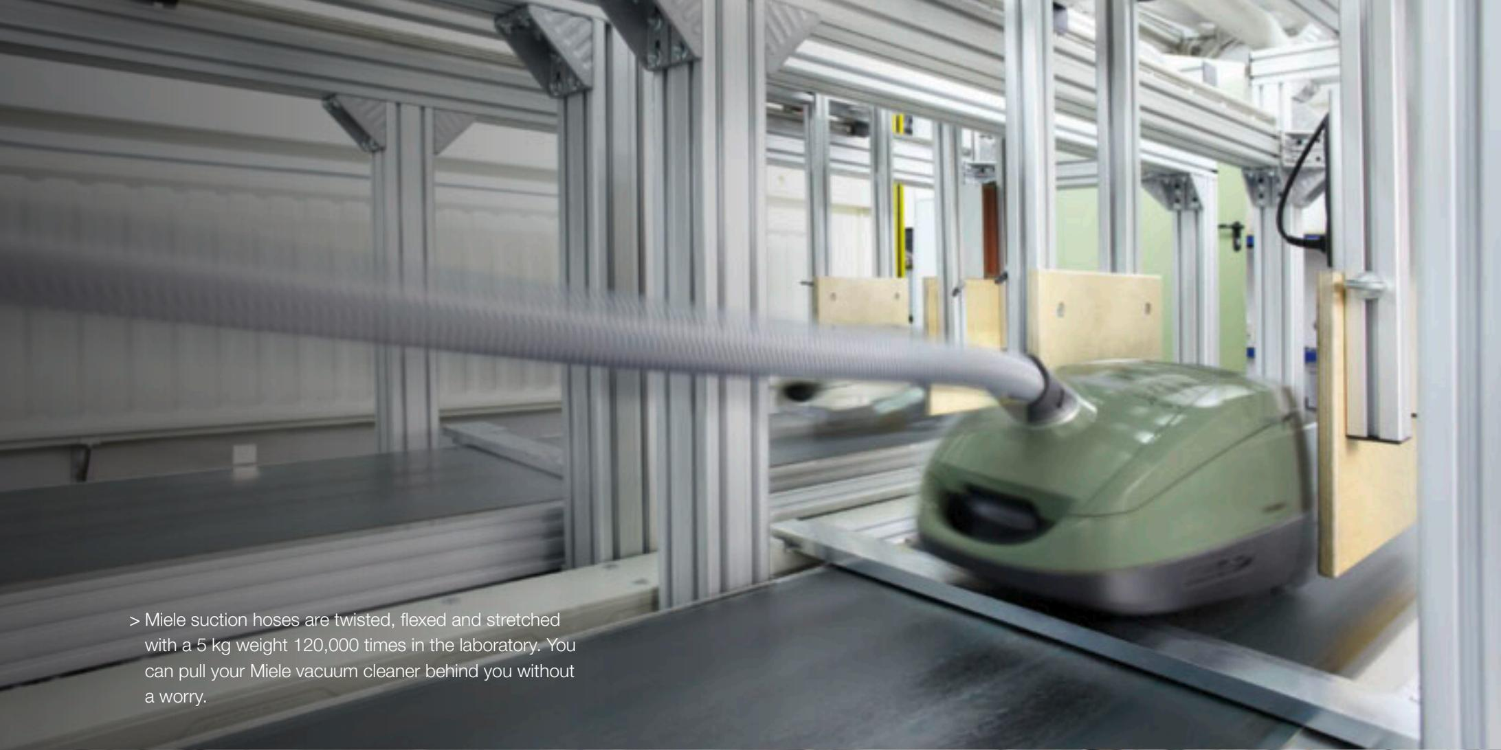
> Miele suction hoses are twisted, flexed and stretched with a 5 kg weight 120,000 times in the laboratory. You can pull your Miele vacuum cleaner behind you without a worry.
