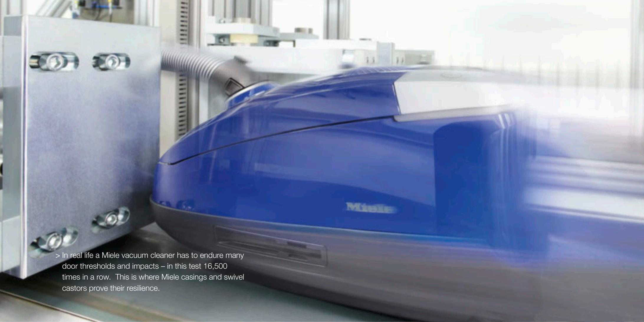
> In real life a Miele vacuum cleaner has to endure many door thresholds and impacts – in this test 16,500 times in a row. This is where Miele casings and swivel castors prove their resilience.
