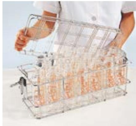
3. After washing and disinfection, the lid is removed and the bottles can be refilled whilst still in the container.
