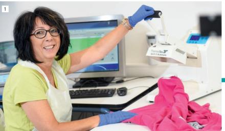
How to save time: Andrea Wallasch (1) patches up new laundry items with the RFID chip. The digital RFID technology from Thermotex makes it possible to trace where exactly an item of laundry has been - for example, when a T-shirt is finished (2). Angelika Wetzel (3) uses the ironing dummy from Veit in order to finish a shirt, which is a much faster method than using a hand iron.
